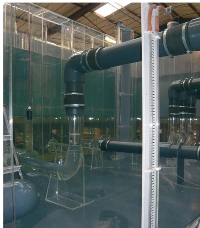
*Perspex Model of Pumping Station*
